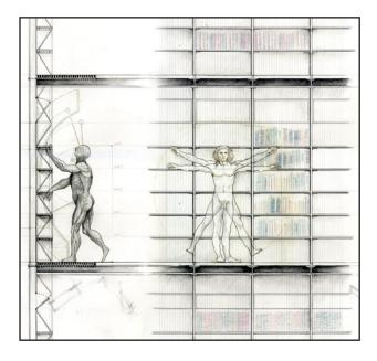
Figure 4: Detail drawing of the bookshelf façade system in relation to bodily interaction and dimensions.
